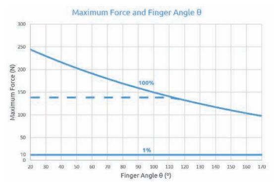
Graph plotted using measurements with 1 A current, silicone fingertips and a metal workpiece. The percetages shown on the graph stand for the target force percentage. The blue line stands for the normal Grip function and the dashed line stands for the Flexible grip function.
